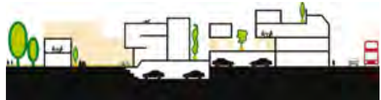
A semi-sunken parking box, with publicly accessible mews deck on top.
